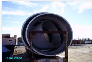
Ductwork Mounted on a Flat Rack container. Approximate weight: 50,000 LBS
