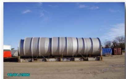
Ductwork before being stripped for final delivery.
